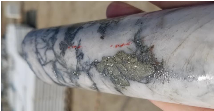
Fig 9. Typical sheeted quartz-sulfide vein mineralization. Pictured includes the interval 161.60 – 161.95m, which assayed 12.90 g/t Au and 203 g/t Ag.*
